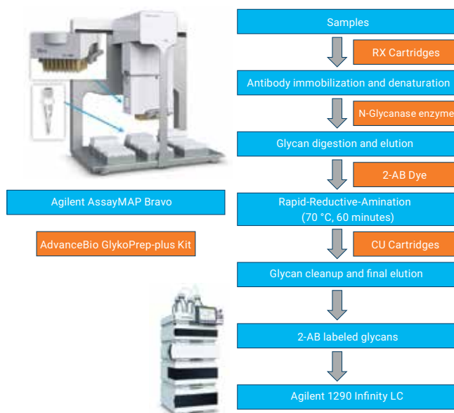
Figure 1. Schematic workflow for the glycan isolation, labelling, purification followed by LC analysis using Agilent solutions. Components of the Agilent AssayMAP steps are shown in blue; the AdvanceBio kits are shown in orange.
